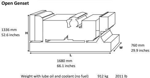
Weight with lube oil and coolant (no fuel) 912 kg
